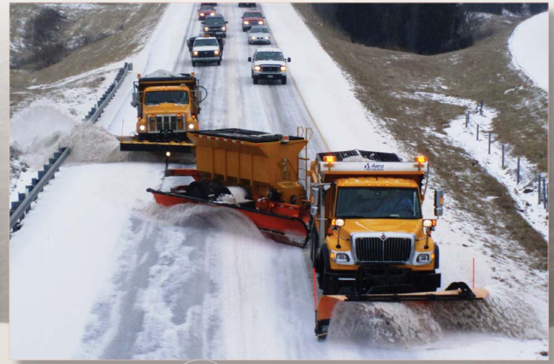
The 26 foot wide, 2-lane Tow Plow is doing winter duty in several States including Ohio, Missouri, Iowa, Utah, Kansas, Maine, Indiana, Wisconsin, Tennessee, Pennsylvania, Nebraska, Colorado
